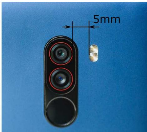
Fig. 1. Camera layout of the Xiaomi Pocophone F1
